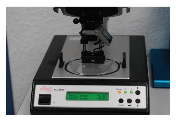
Successful water-resistance test on a SPARC MGS: Both phases, Test 1 at 0.5 bar (= 50 cm) and Test 2 at 10 bar (= 100m/300ft) are indicated with green control-lamps as being passed.
